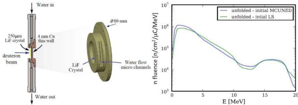
**Figure 13.40:** (Left) A CAD drawing of LiFTiT. Left: transverse cross section. Right: 3D depiction of the LiF crystal and the copper back [1]. (Right) - Unfolded spectra of LiFTiT by using different initial guess spectra. Spectra are normalized to reflect the neutron spectrum at 6 cm distance from the target [1].
