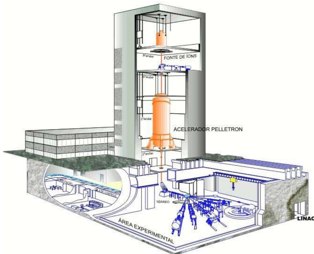
**Figure 15.3:** The 8 UD Pelletron Tandem accelerator.
