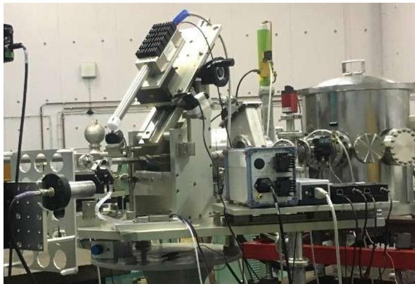
**Figure 13.35:** The RBS/Channeling chamber and the sample manipulator translations and rotations.
