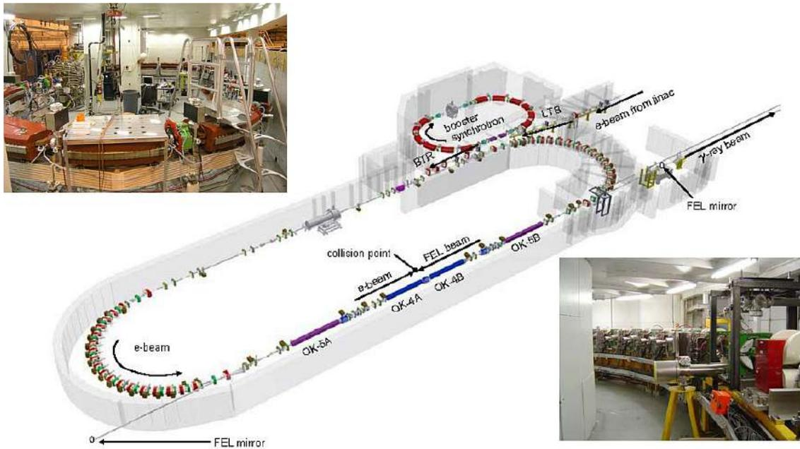
**Figure 14.31:** Layout of the HIGS accelerator systems with photographs of the booster (upper left) and a section of the electron storage ring (lower right).
