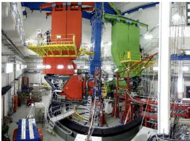
**Figure 13.26:** A1 high resolution spectrometers for electron scattering experiments.
