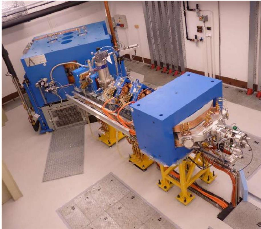
**Figure 13.3:** Photo of the TR-24 Cyclotron.
