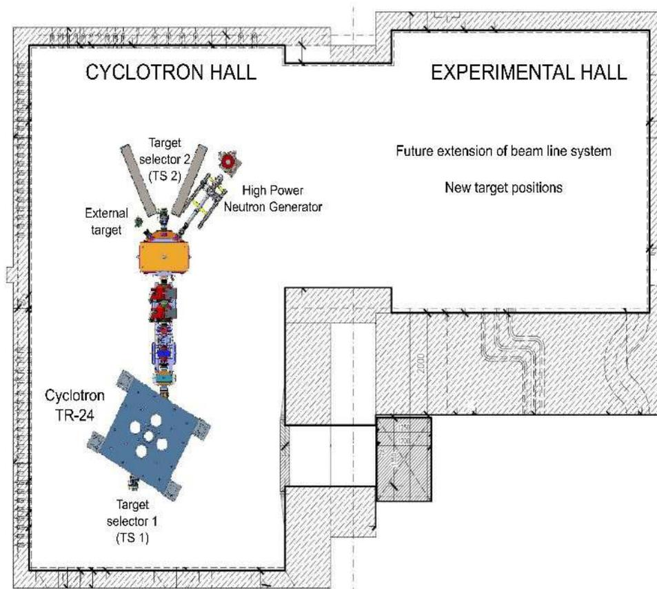
**Figure 13.2:** Layout of the TR-24 Cyclotron.
