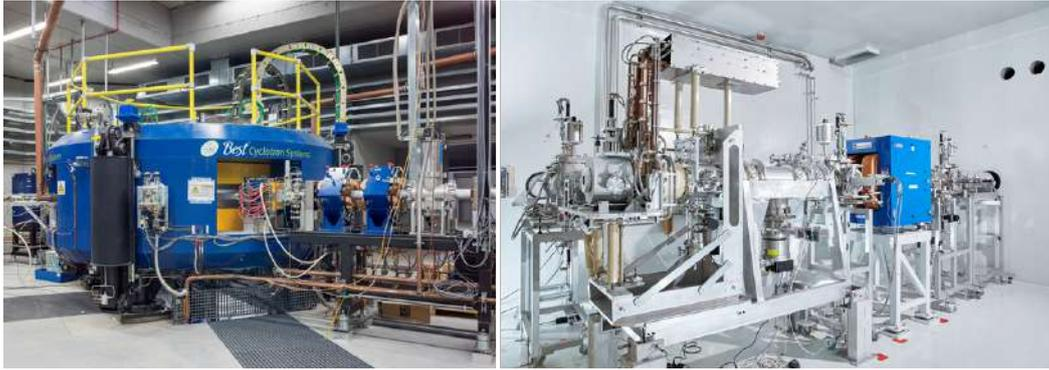
**Figure 13.55:** The cyclotron B70 (left panel) and the ISOL target of SPES (right panel).
