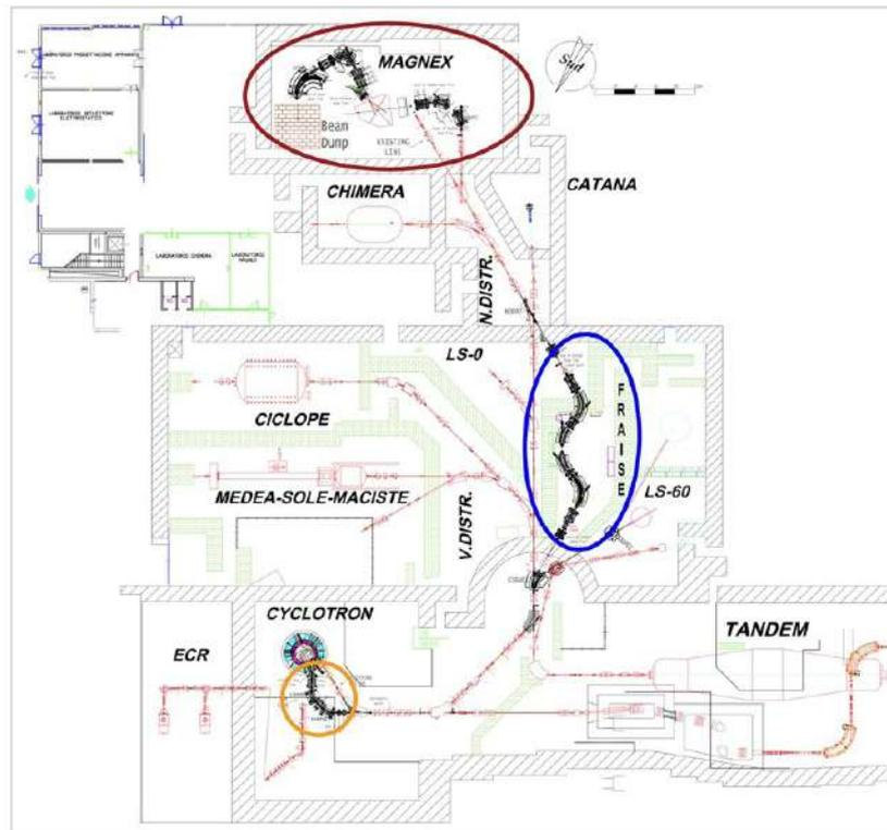
**Figure 13.50:** Schematic layout of LNS beamlines.
