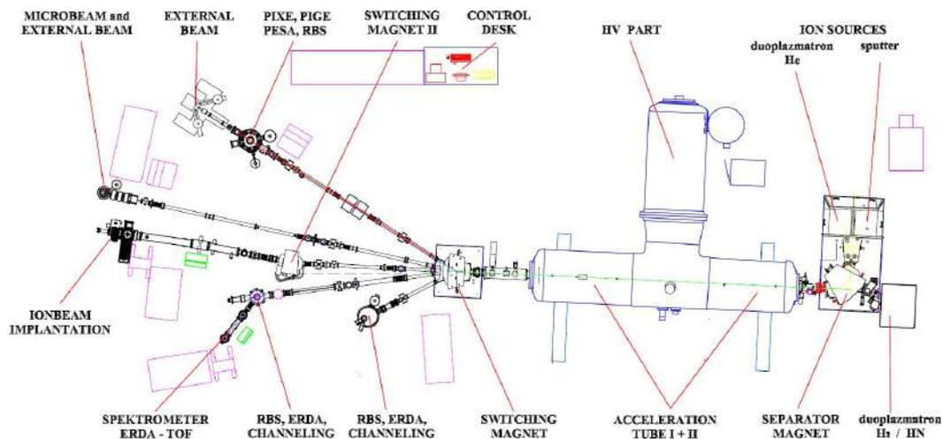
**Figure 13.4:** Layout of the Tandetrion 4130MC.
