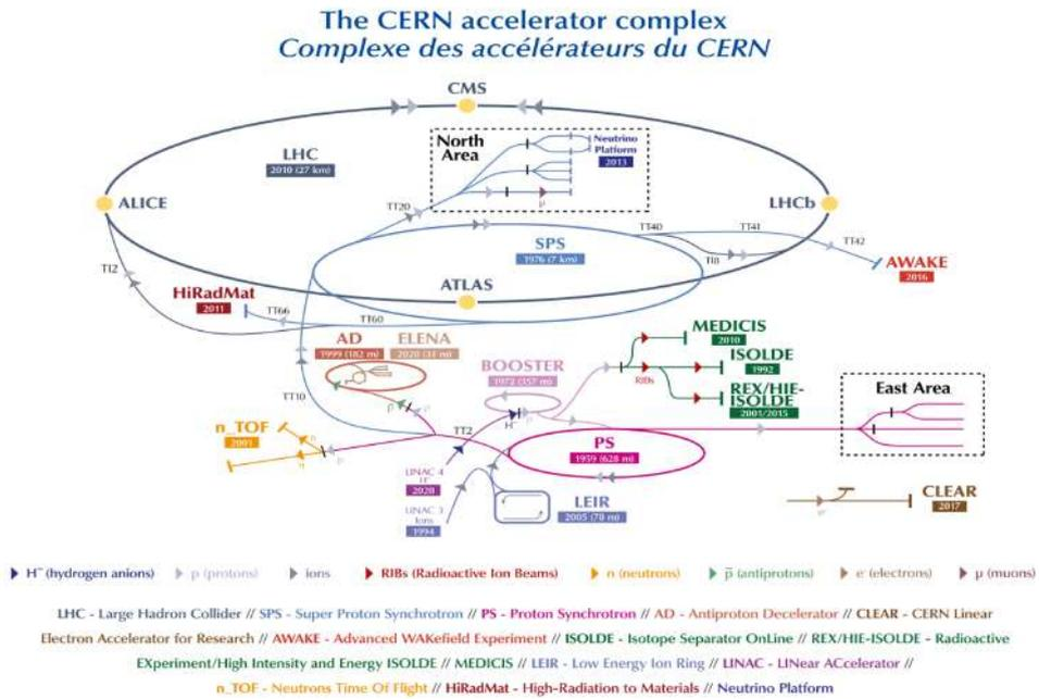
**Figure 13.93:** Accelerator complex at CERN (Image: CERN).
