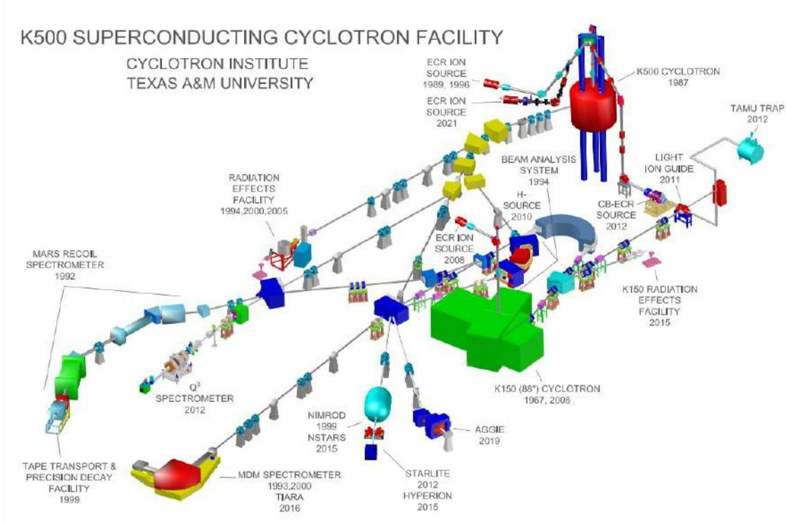
Figure 14.16: Full laboratory layout at the Texas A&M cyclotron.
