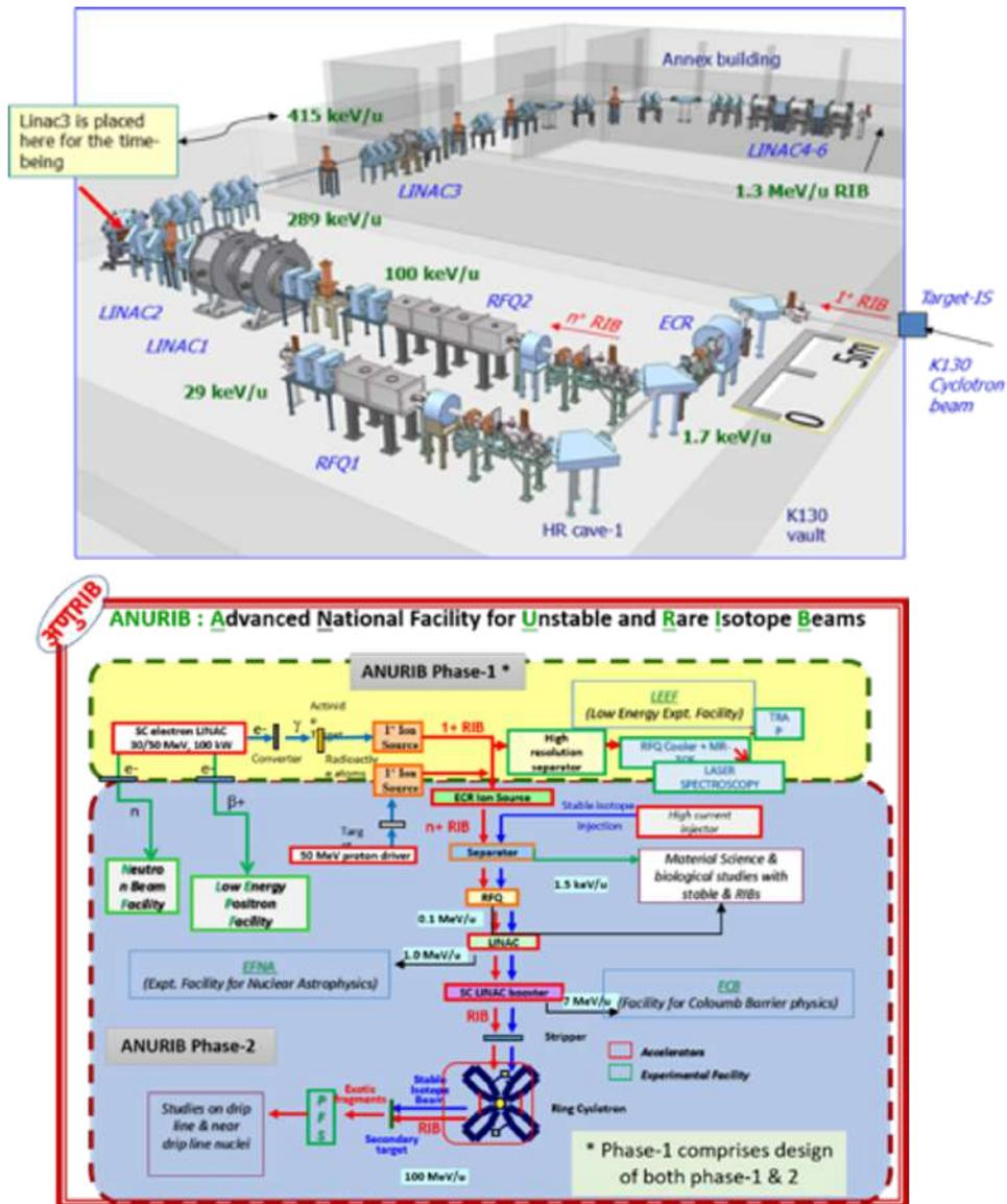
Figure 11.6: RIB facilities at VECC.
