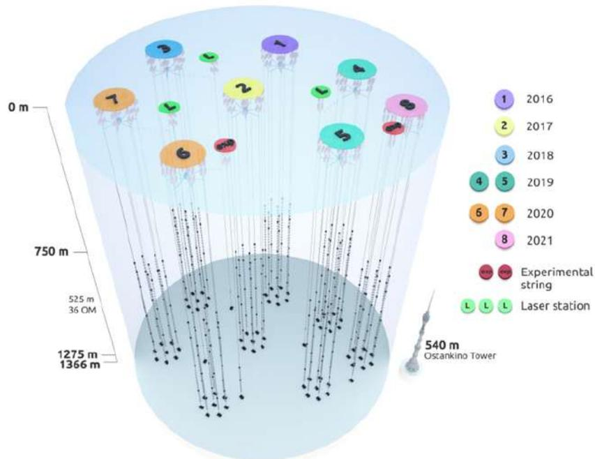
**Figure 13.79:** Baikal-GVD detector.
