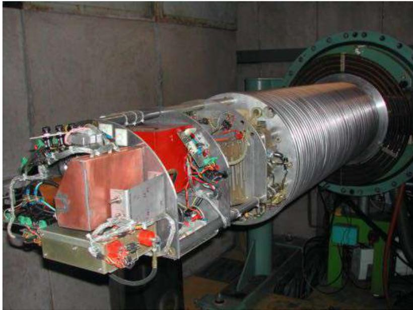
**Figure 13.9:** Van de Graaf 2.5 MV accelerator tube.
