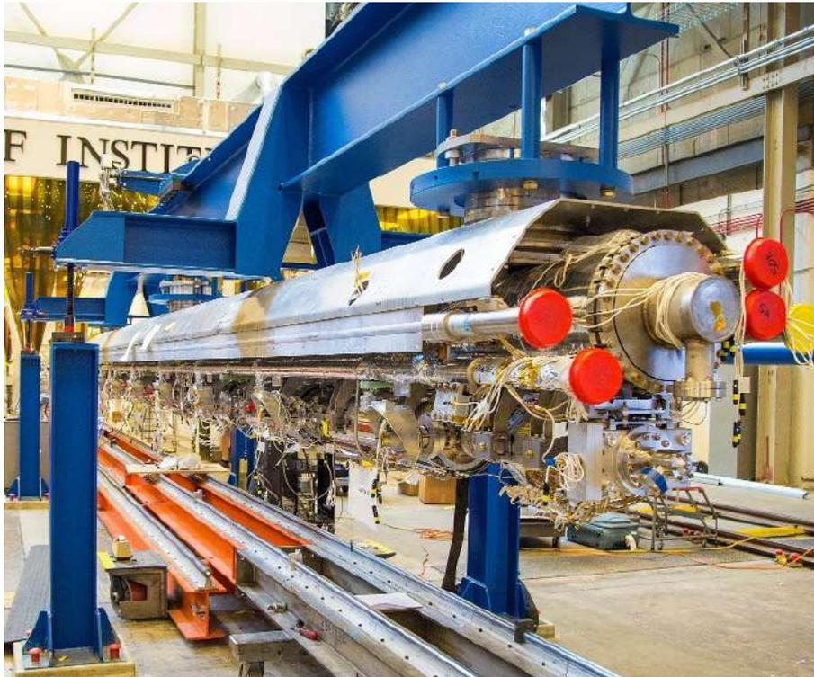
**Figure 14.30:** SRF cryomodule assembly at Jefferson Lab.
