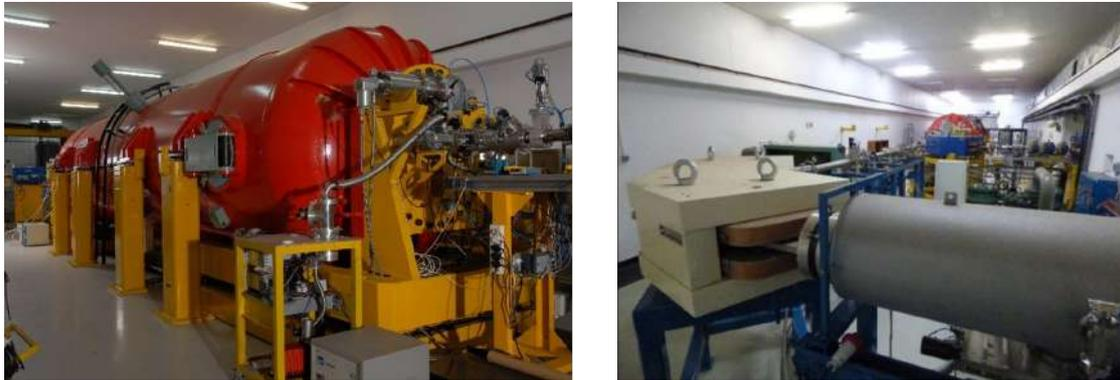
**Figure 10.2:** 6-MV Tandem accelerator (left) and the new bending magnet followed by the electrostatic analyser of the AMS facility (right).
