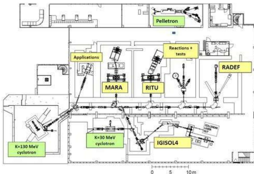
**Figure 13.8:** Layout of the upgraded JYFL Accelerator Laboratory.
