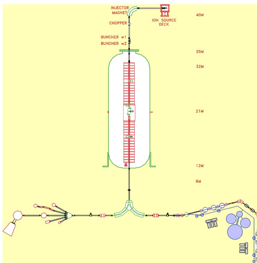
**Figure 11.8:** Schematic layout of 14MV Pelletron accelerator and LINAC
