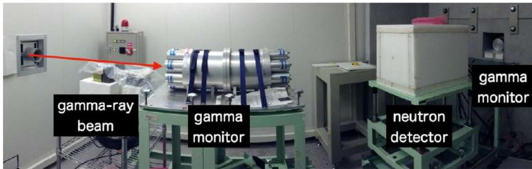
**Figure 11.16:** Photograph of interior of gamma-ray beam irradiation Hutch-2 (GACK)
