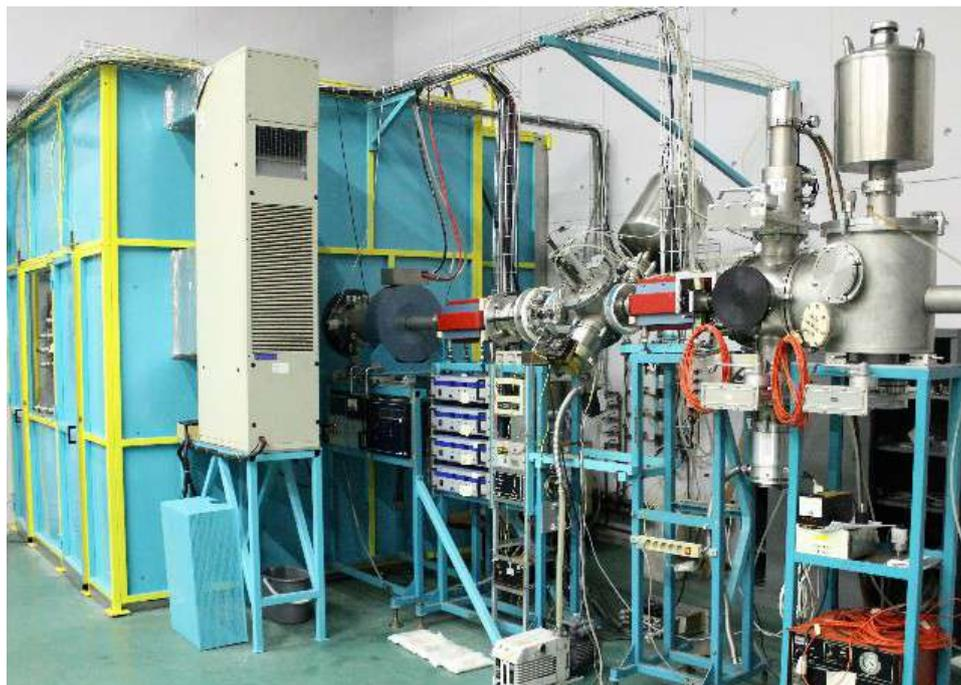
**Figure 13.27:** The single-stage PAPAP accelerator.
