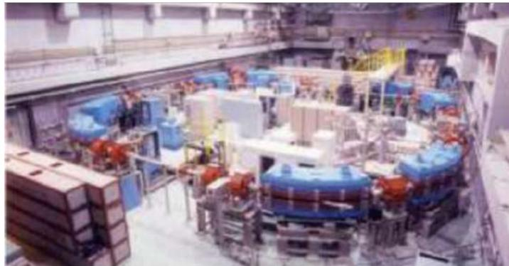
**Figure 11.21:** 1.3 GeV electron booster synchrotron.
