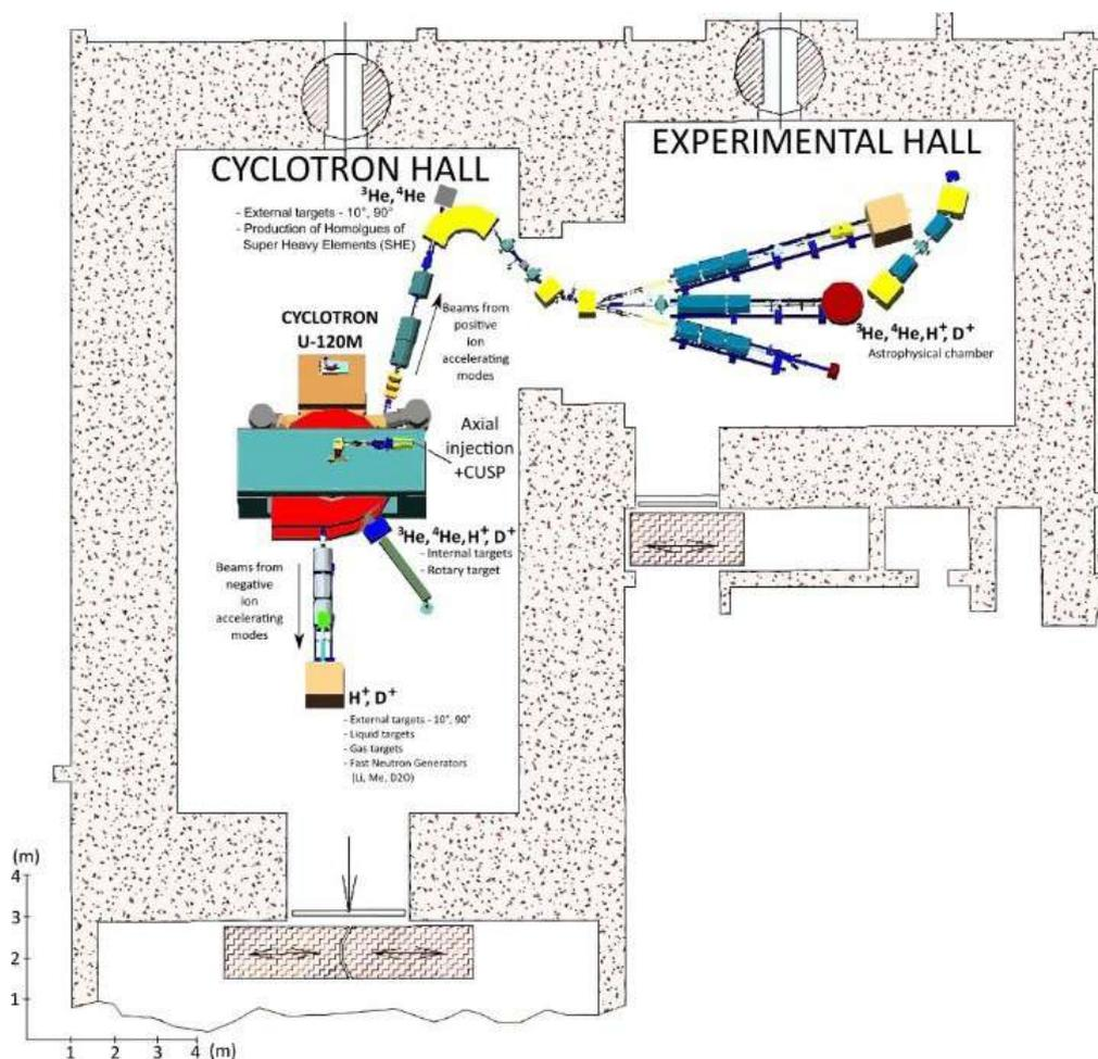
**Figure 13.1:** Layout of the U-120M Isochronous Cyclotron.
