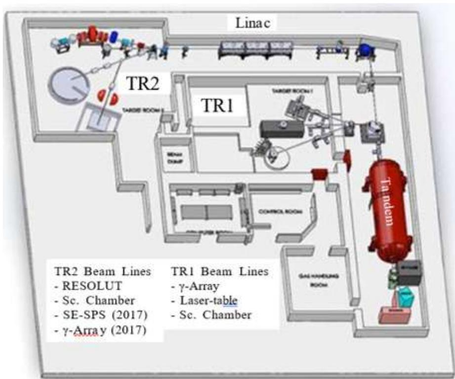
**Figure 14.27:** Accelerator laboratory at Florida State University.
