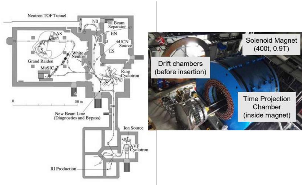
**Figure 11.12:** (Left) Cyclotron facility at JPARC. (Right) LEPS2 Spectrometer.
