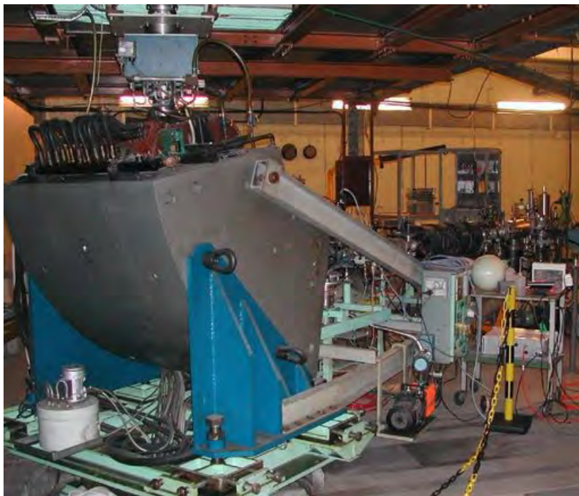
Figure 13.10: Bending magnet of the 4MV Van de Graaff accelerator
