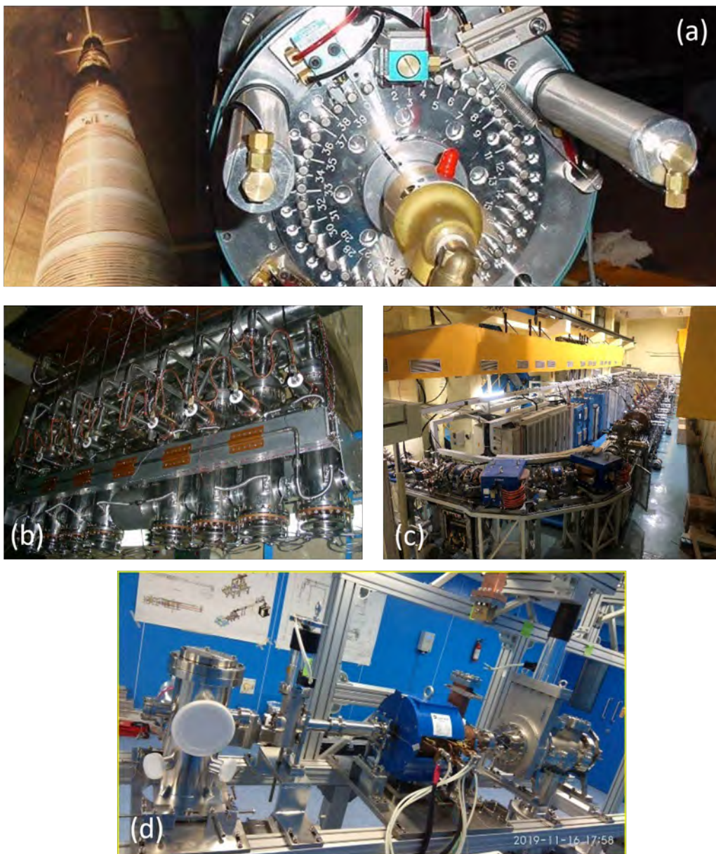
Figure 11.3: Facilities at IUAC: (a) 15 UD Pelletron and SNICS Ion Source; (b) Superconducting Linear Accelerator Module; (c) High Current Injector; (d) Free-electron Laser.
