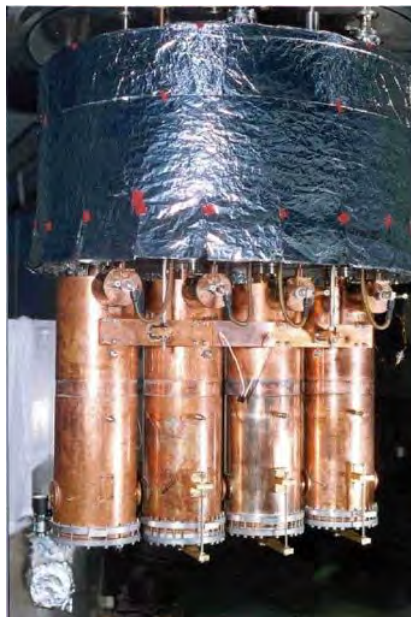
Figure 11.7: Inside view of a LINAC cryostat showing four quarter wave resonators.
