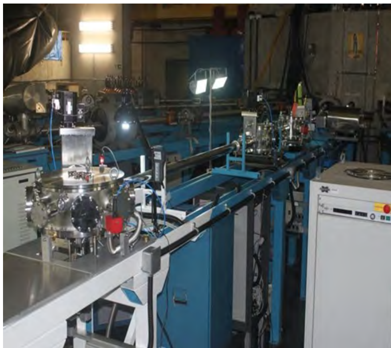
Figure 15.6: The 0 degree beamline composed of three scattering chambers for studies of the effects of radiation in electronic devices.
