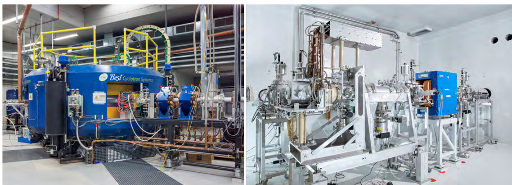
Figure 13.55: The cyclotron B70 (left panel) and the ISOL target of SPES (right panel).
