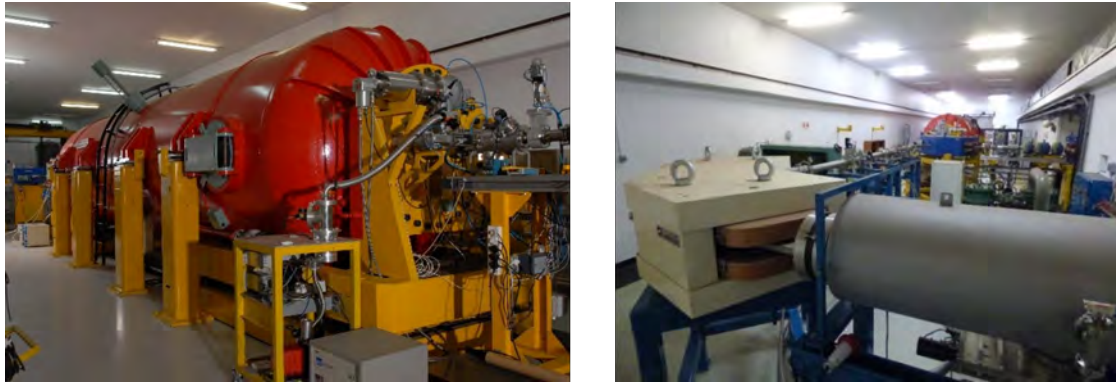
Figure 10.2: 6-MV Tandem accelerator (left) and the new bending magnet followed by the electrostatic analyser of the AMS facility (right).
